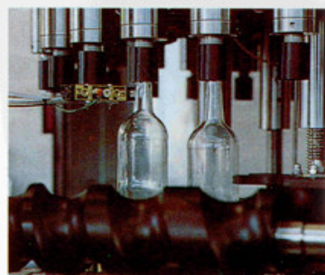
BOTTLE CONVEYOR SYSTEM
