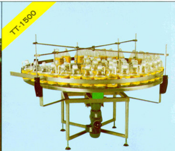
Motorised turntable for connection to the filling machine to continuously feed containers to the infeed conveyor. It can also be connected to the end of conveyor to collect filling and capped containers.
