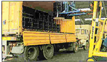
Container loaded in 20-30 minutes using 2-drum standard Grab-O-Matic with Long Reach attachment.
